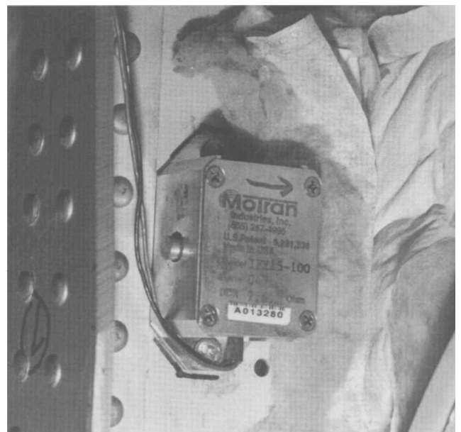
Fig. 6 Inertial actuator mounted to 1900D frame.
